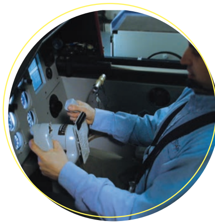
The GYROLAB GL-2000 simulator replicates the dynamics of an upset condition.
