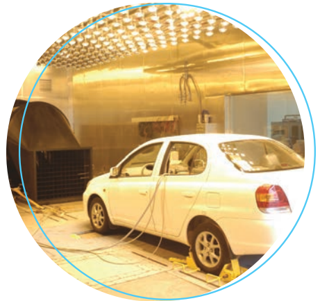
ETC Testing & Simulation Systems Drive-In Test Chamber
